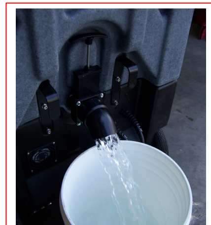
Drain water from Recovery Tank
