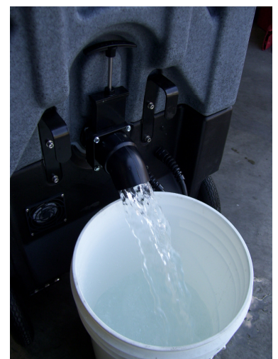
Draining the Recovery Tank
