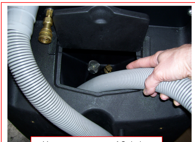
Vacuum water out of Solution Tank
